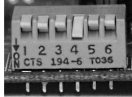
If you wish to eliminate the 3-second requirement for HF cycler activation and have it activated immediately when the vehicle horn is pressed, set DIP switch #4 into the DOWN (On) position (as pictured above).
